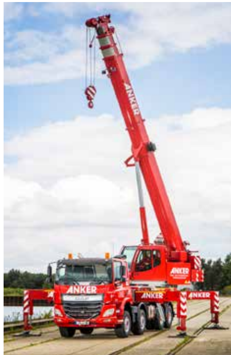
The 8x4 CF vehicles with sleeper cabin have a crane configuration with a reach of no less than 35.20 metres, and a lifting capacity of 40 tonnes.
