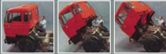
The tilt construction was a textbook example of the creativity of the DAF developers.
