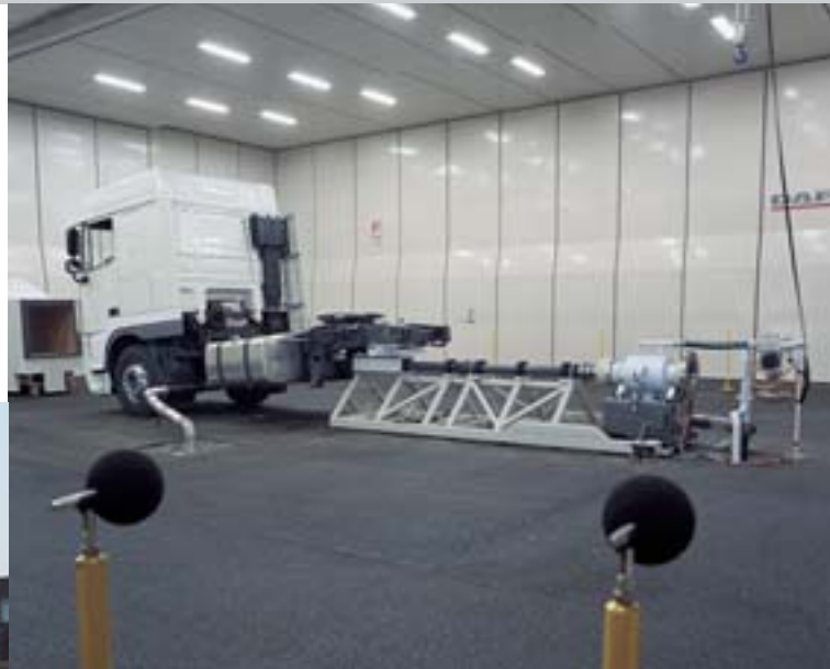
Above: On the left the driving wind simulator, in the middle the vehicle to be tested and at the back the water brake, which during tests loads the driveline as if the truck were driving on the road. In the foreground, two extremely sensitive microphones.
