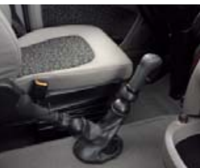
Retractable gear lever for unhindered movement in the cab.
