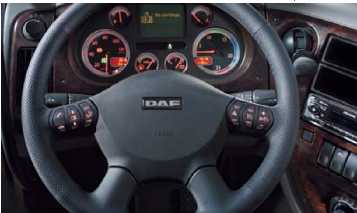
The new steering wheel can be delivered with integrated switches for cruise control, down hill speed control and telephone, etc.
