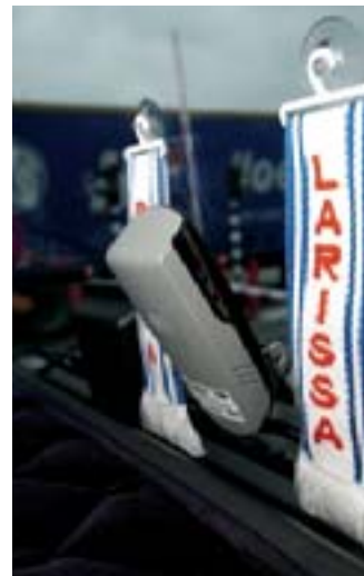
According to the BAG, drivers place objects all too often around the sensor in front of the windscreen causing malfunctions as a result.
